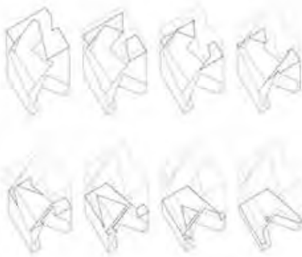
diagram of layered pouring of plaster
